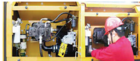
Replace diesel oil filter element
