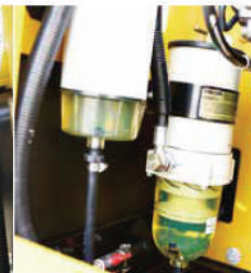
Water drain valve and check valve of fuel tank
