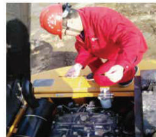
Inspect the situation of engine oil
