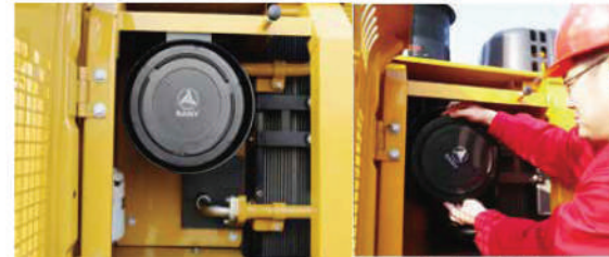
Replace air filter element
